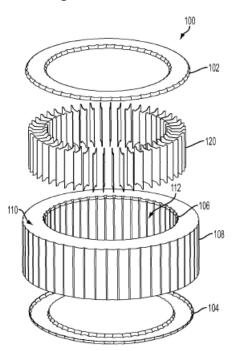
Figure 1 is an exploded perspective view of an inflatable spa, including tensioning structures. Ex. 1001, 4:27–29. The inflatable spa 100 has internal wall 106 and external wall 108 that together, along with top and bottom walls (102 and 104, respectively), define inflatable air chamber 110. *Id.* at 5:60–6:9. Tensioning structures 120 couple the inner and outer walls, and may have gaps at the top and bottom. *Id.* at 6:30–38.
