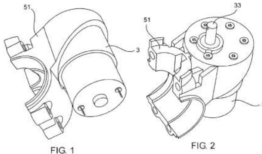
Figures 1 and 2 illustrate “the motor (3) whereby it is attached to the inner clamp (5).” *Id.* at 1:52–53; *see id.* at 2:42–43.
