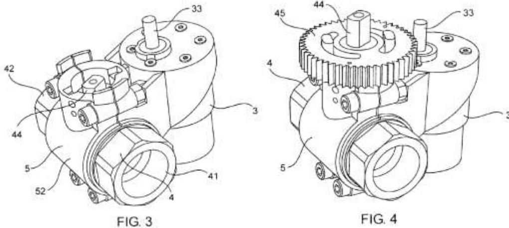
Figures 3 and 4 “depict the electric motor (3) whereby it is attached to the inner clamp (5), into which the inner pipe (4) is inserted.” *Id.* at 1:54–56.
