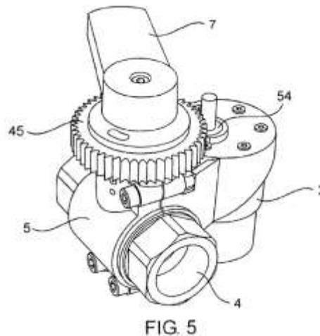
Figure 5 “depicts the electric motor (3), the inner clamp (5), the inner pipe (4), the motor axle (33), the rotation shaft (44), the secondary cogwheel (45), and the manual handle (7).” *Id.* at 1:57–59; *see id.* at 2:57–59.
