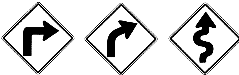
187: Many traffic signs communicate through an iconic resemblance to a given class of roadway feature. The high degree of abstraction is essential for both generality (the sign can refer to any similar curve) and recognizability.
