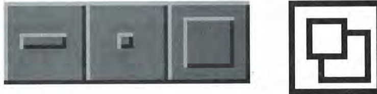
196: Generalized imagery is used throughout the GUI environment to represent standard control and feedback mechanisms. These examples from the OSF/Motif (a) and Macintosh (b) standards, are abstract symbols depending on constant exposure to ensure their understandability.
