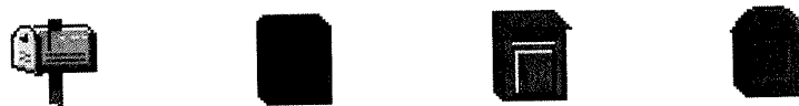
207: Cultural dependency is apparent in these icons representing mailboxes in the U.S. (a), Denmark (b), France (c), and Italy (d). Each could be interpreted as a control box or trash can by someone unfamiliar with the local convention. Line art is the property of Apple Computer, Inc.
