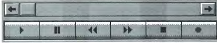
195: Simple, abstract representations such as these standard transport control symbols are generalizable not only across software applications, but across hardware platforms and product categories (e.g., consumer electronics) as well. They are widely understood when used consistently.
