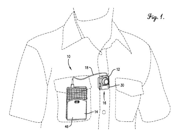
Figure 1 depicts an embodiment of the '730 patent in the form of a portable video and imaging system mounted on a user's body. *Id.* at 2:41–43. As shown in Figure 1 above, digital video recording system 10 comprises camera component 12, recording component 14, and mounting assembly 16. *Id.* at 4:39–42.
