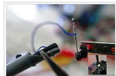
Green electroluminescence from a point contact on a crystal of SiC recreates H. J. Round's original experiment from 1907.
