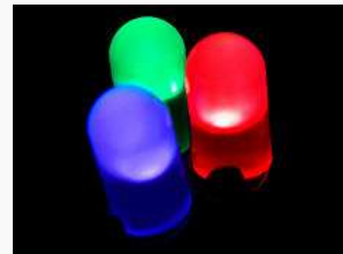
Red, pure green and blue LEDs of the 5mm diffused type
