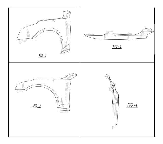
Ex. 1001. Figures 1–4 above are line drawings that depict, respectively, a front and left perspective view, a top plan view, a left end elevation view, and a front elevation view of the claimed vehicle bumper design. *Id.* (57).
