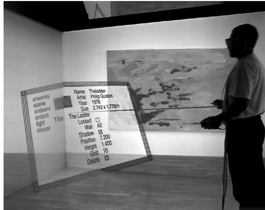
Figure 8.2 A floating menu in the Virtual Museum application. (Photograph courtesy of Gerhard Eckel, Fraunhofer IMK)
