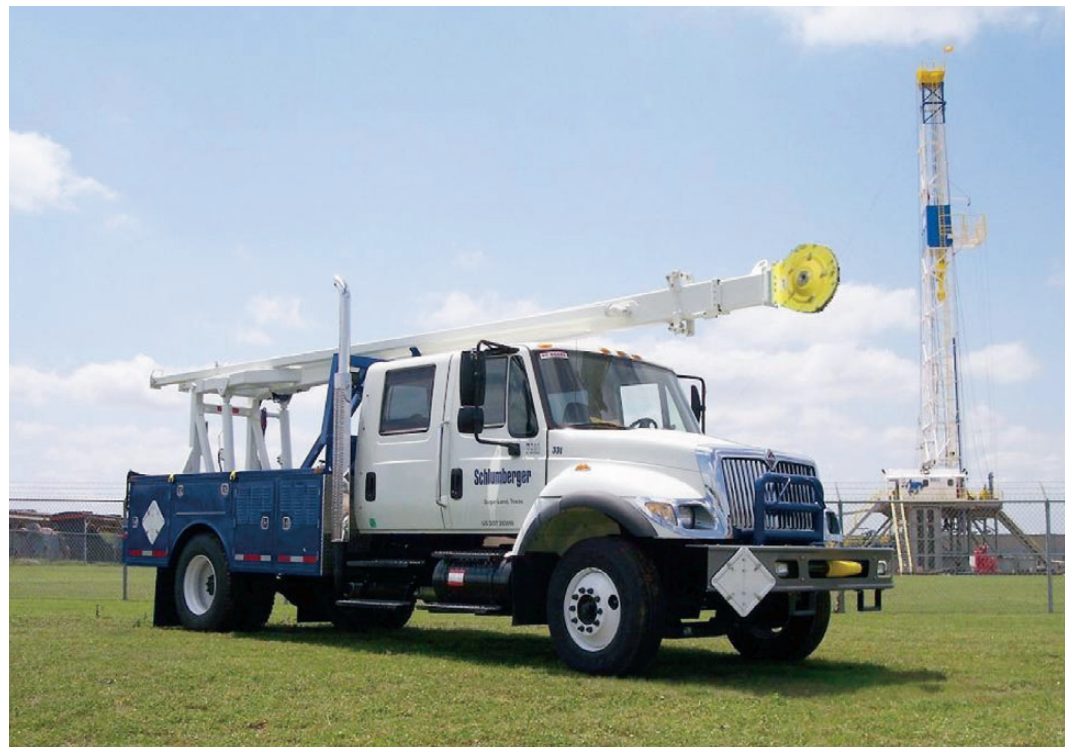
Figure 192. SWPT-GAB on a 4 × 2 chassis with integral mast.
