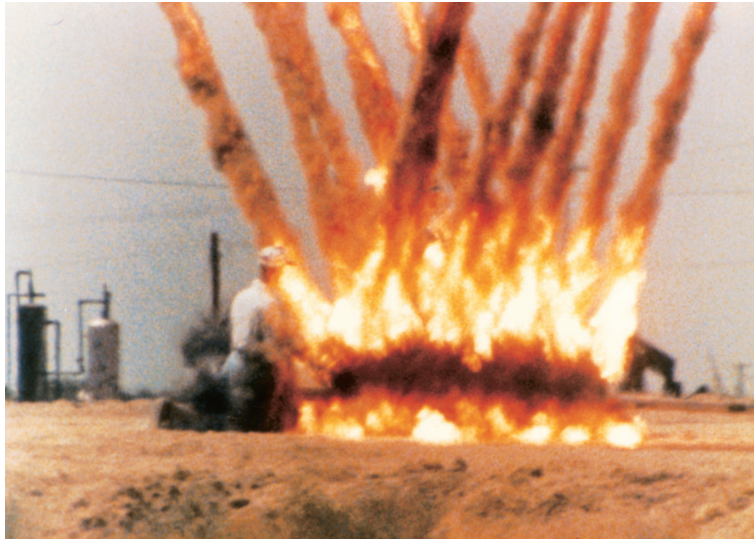
Figure 1. A perforating gun detonated at the surface demonstrates the tremendous power of an oilwell perforator. The figure at left is a mannequin.
