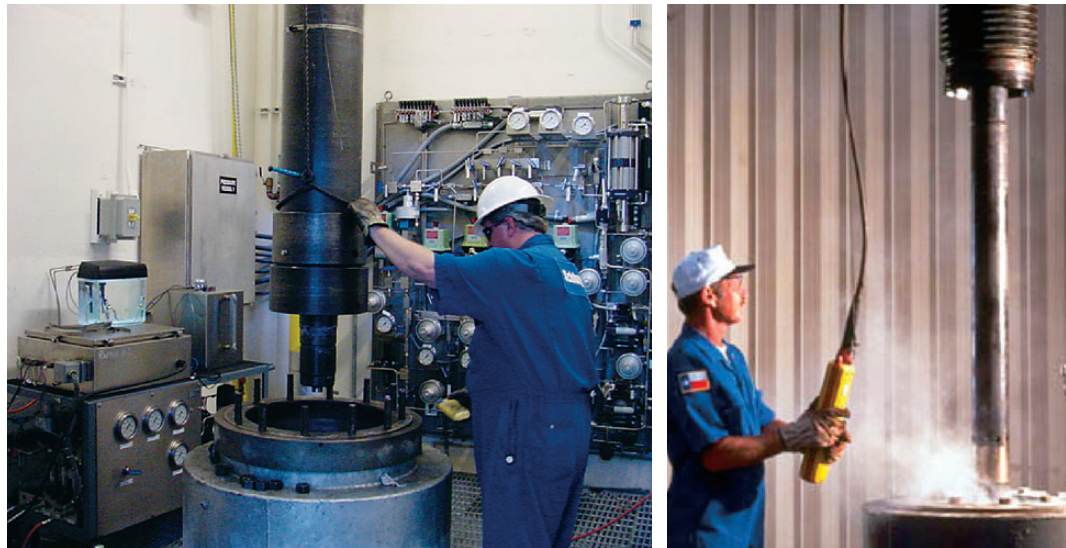
Figure 197. Qualification setup for the MAXR automatic release anchor.
