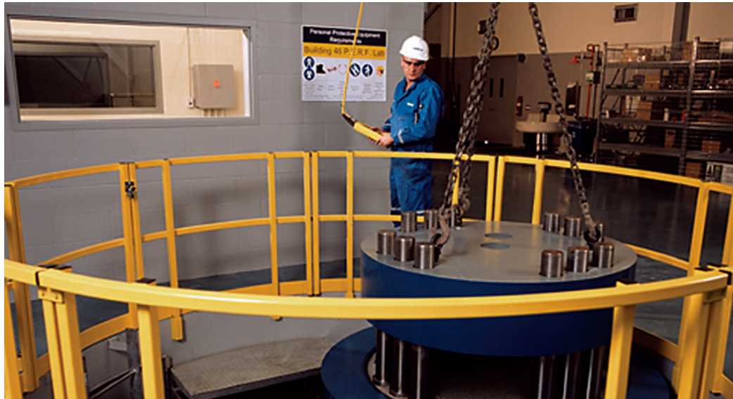
Figure 90. Installation of the top steel platen onto the 12 tie rods of the assembled polyaxial stress frame.
