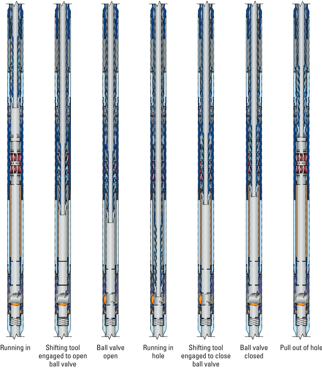
Figure 342. FIV shifting tool positions.
