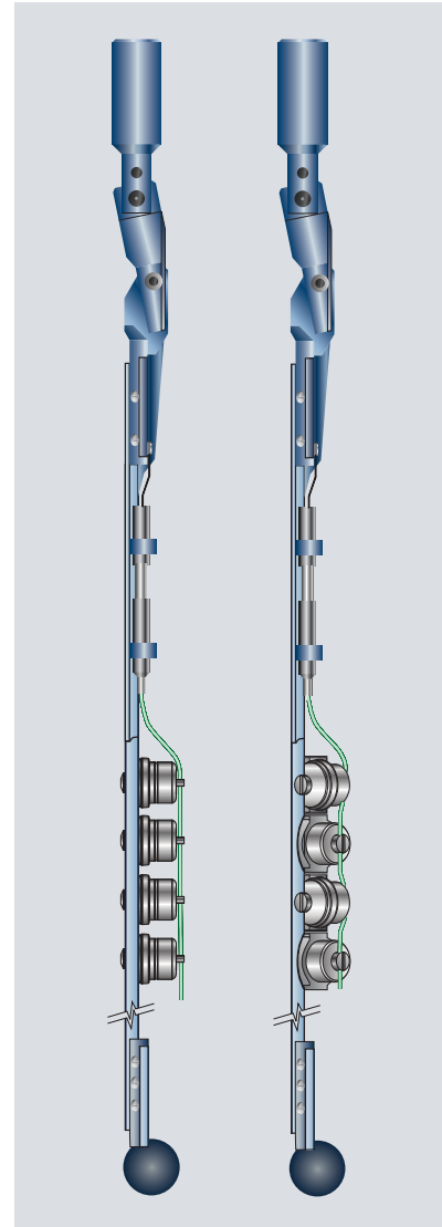
Figure 103. 1 11 / 16 -in. retrievable Enerjet gun.
