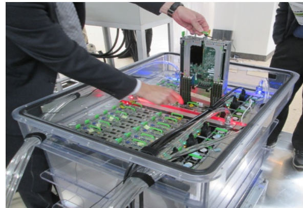
Fig. 4. Snap shot of liquid immersion system with natural convection.
