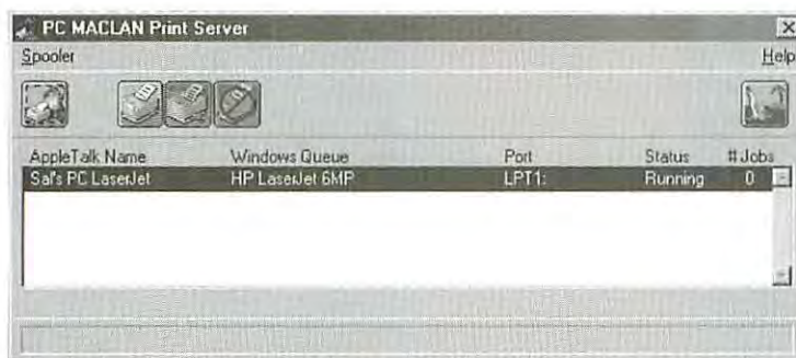
PC MACLAN's Print Server makes PostScript printers connected to PCs available on Macs.
