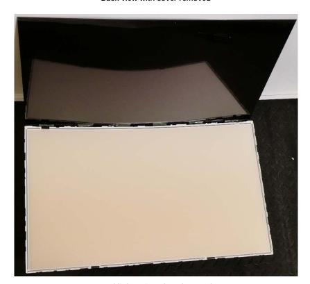
Backlight unit under LCD panel
