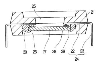
The patent explains that the larger size of opening 26 allows chip 27 to be inserted into the package 21 through opening 26, positioned, and then fixed in place. *See id.* at col. 5 ll. 9–22.
