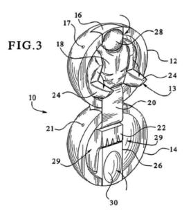
In Figure 3, the head, or first revealer 16, has rotated around, so that the image of the face is in the "concealed position." *Id.* at col. 3, line 57, through col. 4, line 6. The arms, or second revealers 24, have been retracted downward from their extended position shown in Figure 1. *Id.* at col. 4, ll. 18–24. Finally, the third revealer 26, which constitutes the feet of the figurine, has been moved up to a concealed position. *Id.* at col. 4, ll. 40–59.
