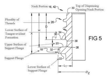
J.A. 5305. The X dimension in Figure 5 (delineated by the vertical line to the far left of the diagram) represents a measurement of the vertical distance from the top of the dispensing opening/neck portion (30) to the lower surface of the support flange (22), including the threads and a TEF. Decreasing the magnitude of the X dimension can result in lighter weight bottles and preforms, with related economic and manufacturing benefits.
