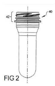
(Def.'s PFOFs (dkt. #107) ¶ 41.) A preform includes a neck portion (often referred to as a "neck finish"), indicated by reference number 42 above, and beneath the neck portion, a lower portion that resembles a test tube.
