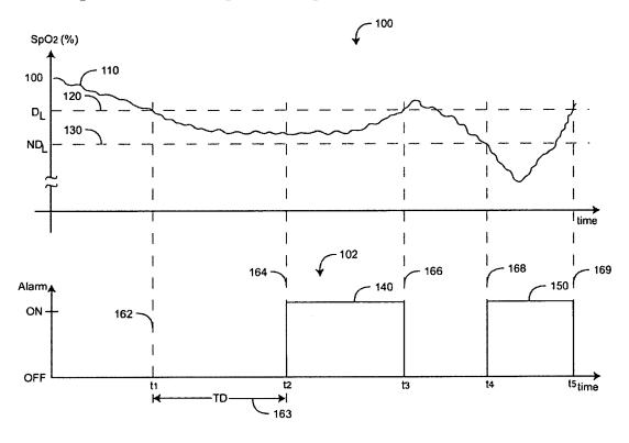
Figure 1 illustrates a prior art oxygen saturation measurement system having two "lower-limit, *fixed-threshold* alarm" schemes, at "delay" alarm threshold  $D_L$  and at "no delay" alarm threshold  $ND_L$ . *Id.* at 2:54–59 (emphasis added). If the patient's measured oxygen saturation 110 falls and stays below delay threshold  $D_L$  for a time period greater than time delay TD,
